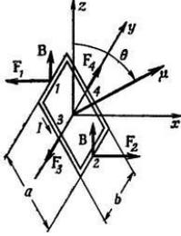
Fig.3. Frame with current in a magnetic field
